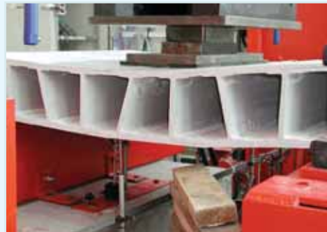
DuraSpan transverse bending test — North Carolina State University
