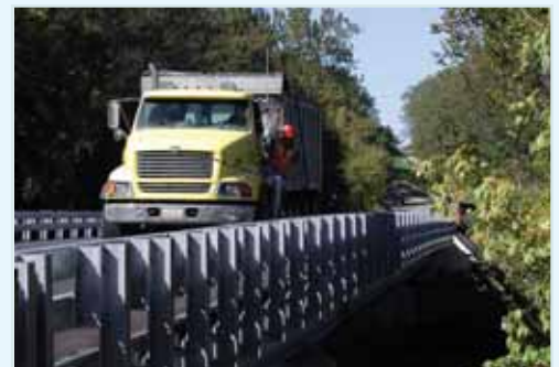
Field load testing — Greene County, Ohio
