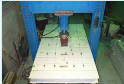
Effective width/composite action test — University of Pittsburgh
